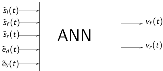
Figure: 3 layer feed forward ANN controller. 5 inputs and 2 outputs. \tilde{s}_l(t) , \tilde{s}_f(t) and \tilde{s}_r(t) represent the average obstacle presence to the left, front and right of the robot. \tilde{e}_\theta(t) and \tilde{e}_d(t) are the normalized distance and angle error. Tilde on the input variables denote that these are the normalized values. 1 hidden layer with 10 neurons. Output neurons are linear and hidden neurons use a scaled tanh() non-linear activation function.
